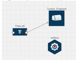
Figure 20 Adding a link from Pass-all Map to Tunnel\_Endpoint
